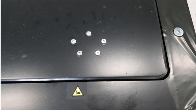
If you are having difficulty screwing in the short bolts, start by using a long bolt to make the others easier to screw in. Remember to replace the long bolt with a short one when you are finished. You can also widen the holes using a hex key or other tool.
