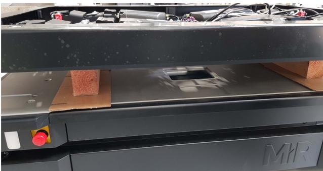
2. Lower the lift onto the robot.
