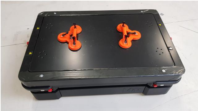
9. Screw in all twenty screws to fix the cover to the lifting device. Ensure the screws are plane with the lift cover.
