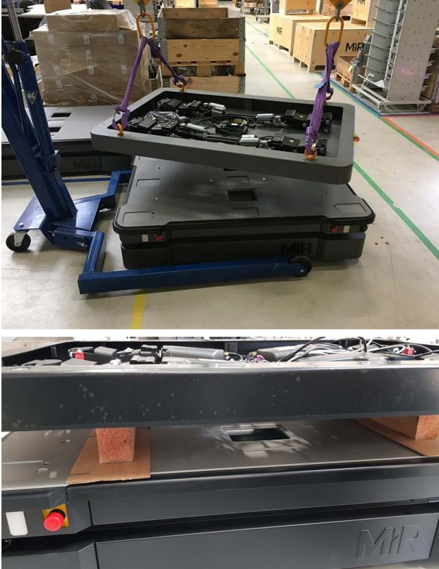
5. Remove the cables from the bag. Notice that there are two cables for each side of the lifting device. Feed the cables through the hole on the right side and vice versa with the left side.
